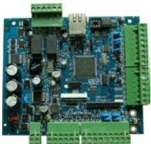
Lift controller Model : CTRL-1DRLIFT-CF/IP(2.0A)-PCB
